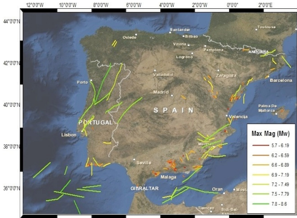
Figure 4. Map showing maximum magnitude (M w ) for composite seismogenic sources (CSS) in Iberia.
